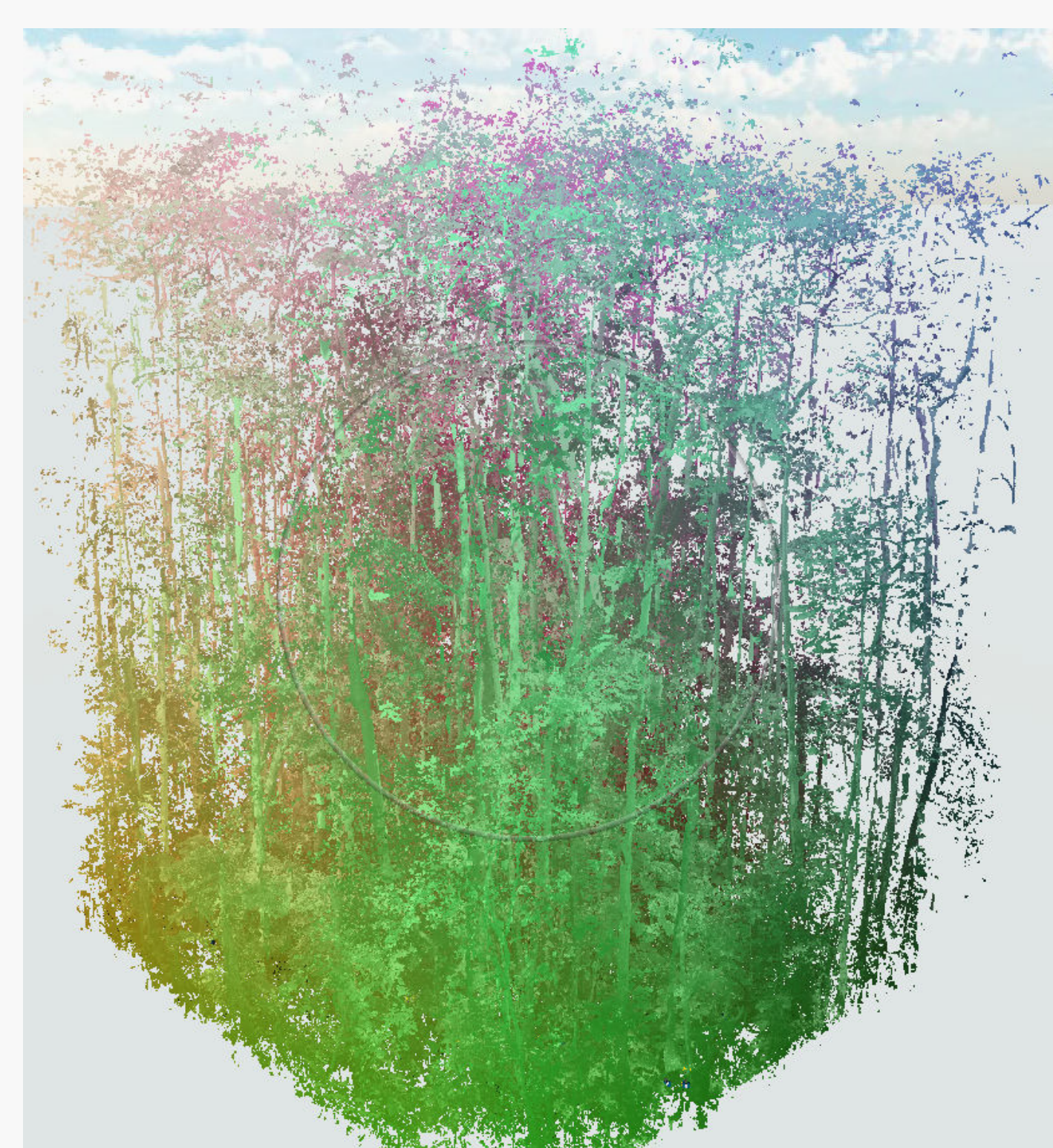
Fig. 7: Leaf-on forest point cloud of 25x25m 2 plot in the swamp forest of Hlanzoun, Benin. The point cloud is colored according to x-, y-, and z-axis.
