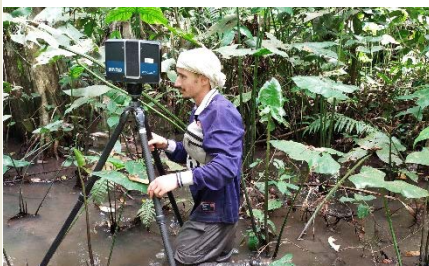
Fig. 4: Samuel Hepner using terrestrial laser scanner in Lokoli swamp forest, Benin.
